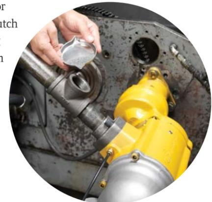
**Brutal lab testing featuring steel shot in the starter's inlet line demonstrates the ST1000's rugged reliability**
