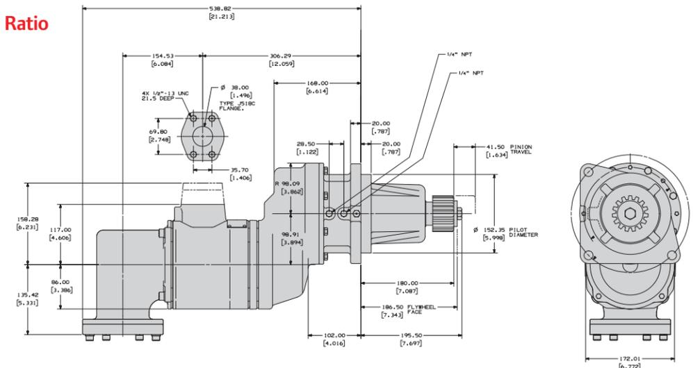
Note: Illustrations not to scale. Dimensions in mm (in). Elbow exhaust shown for pre-engaged models, but straight exhaust is also available. Elbow exhaust configuration is also available for the inertia starter shown above.
